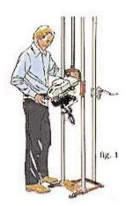
Assembly of the Power Mast takes only a few minutes and is completed by placing the engine into the cradle (fig.1).
