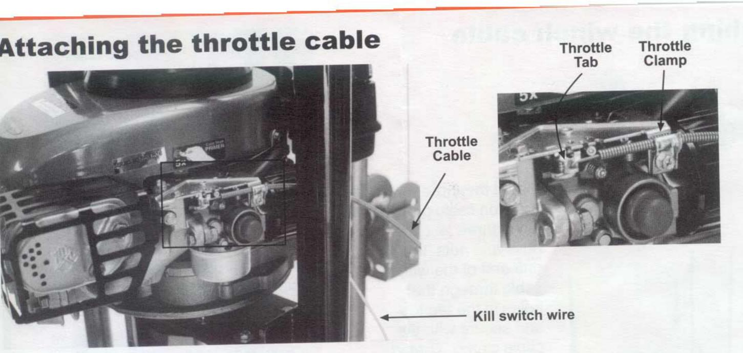
Insert the end of the throttle cable through the throttle tab on the engine, then lay the cable into the clamp and secure with the clamp screw. Operate the throttle control above the winch to be sure the throttle tab swings freely back and forth.
