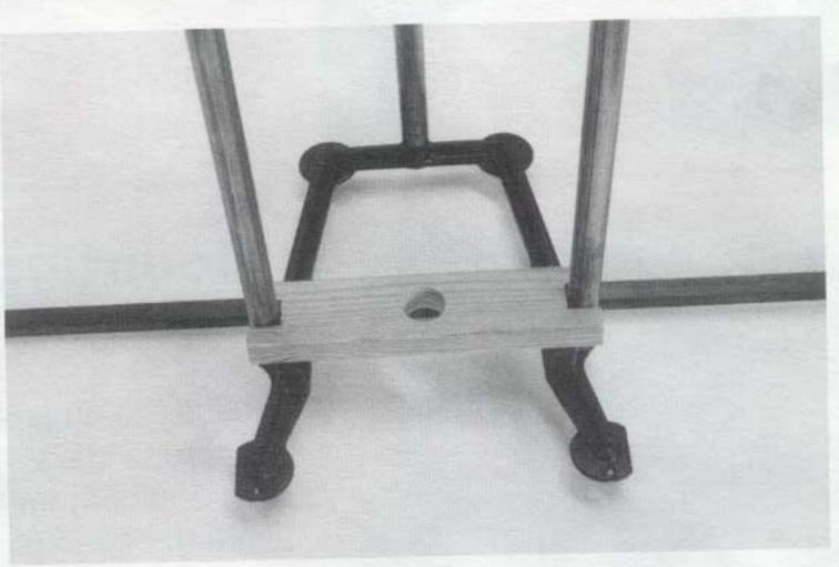
Place the drill stem guide onto the poles and base.
