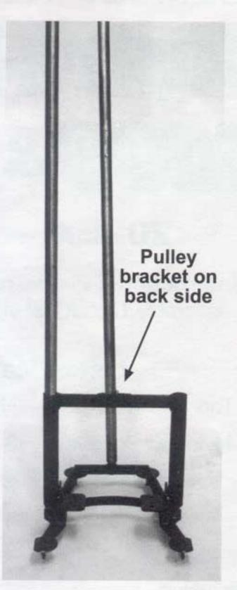
Place the engine cradle onto the front posts of the base. The pulley bracket goes to the rear. Insert the two front poles through the cradle and onto the base posts.
