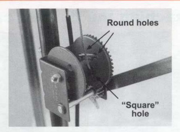
Insert the winch cable from inside reel to outside through "square" hole. Push cable into one of the round holes, then out through the other round hole.
