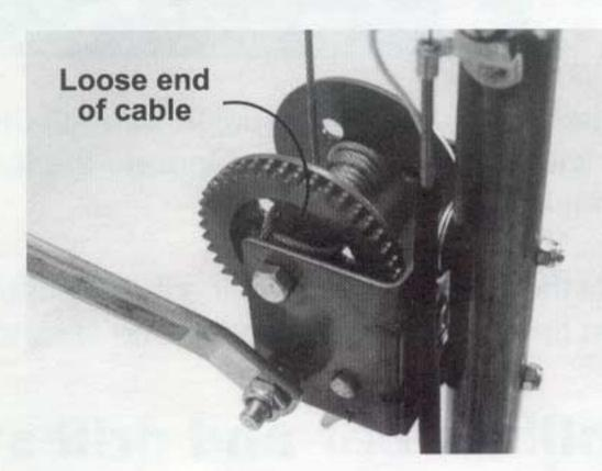
Slip the end of the cable under the loop to hold taut. Hold some tension against the cable and crank it onto the winch, taking out all the slack.
